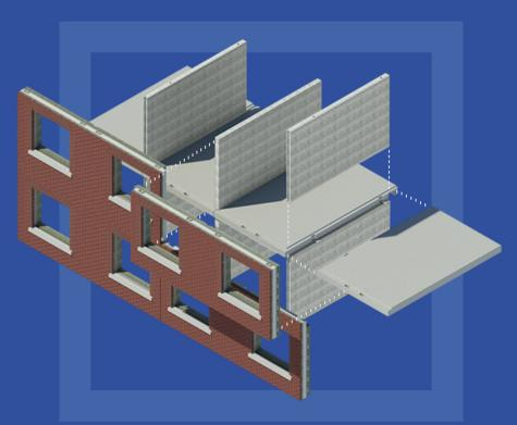
Systemised DfMA delivery of accommodation structures and façades. An Offsite system build 'kit of parts' approach which delivers modern functional living spaces with inherent fire and sound resistance, low operational energy requirements which provides excellent client value.
